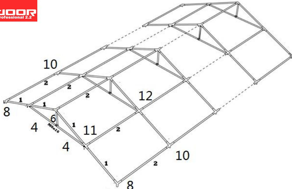
Select a flat ground for the tent, unpack each carton, and check all parts are present. Display all parts as on the drawing
